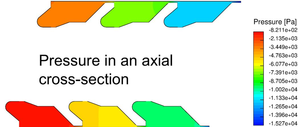
**Fully developed flow assumed – periodic boundary conditions at inlet and outlet, computation in a rotating frame of reference...**
