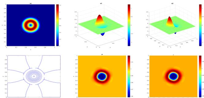
Upper figures: velocity magnitude and components; bellow: streamlines, pressure and density
